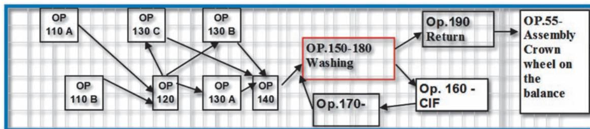
**Figure 2** – The manufacturing process of the crown wheel
