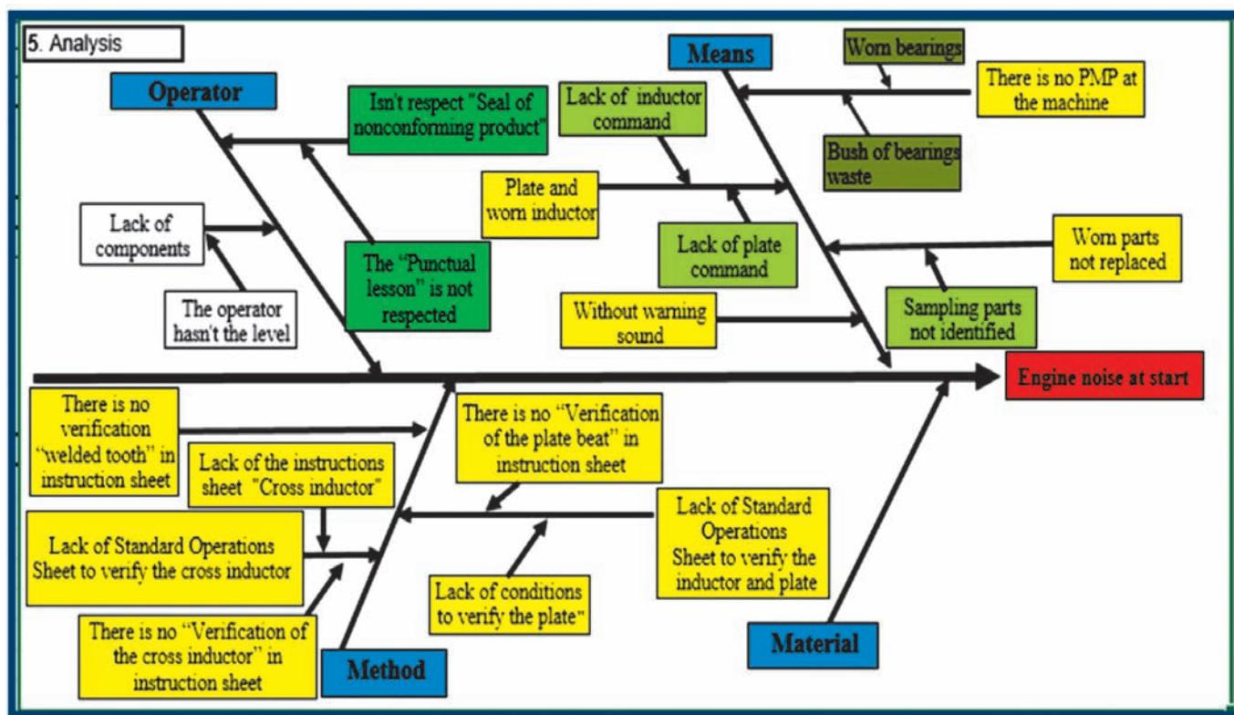
**Figure 4 – Ishikawa diagram for „engine noise at start” failure**
