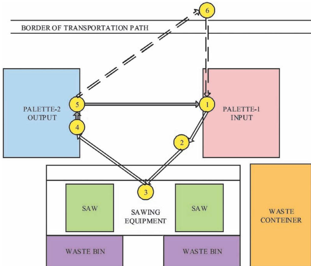
**Figure 1** – Workstation scheme and working sequence in it
