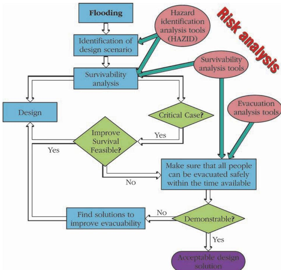
Figure 4 – Risk based design iteration process
