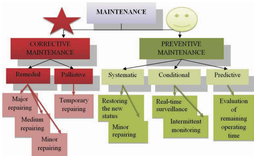
**Figure 2** – The components of the maintenance system and the basic maintenance activities
