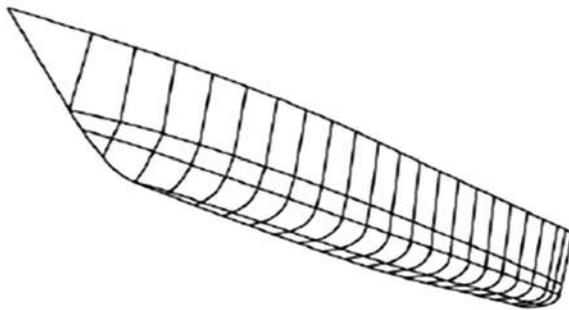
**Figure 7** – *Grid definition and resulting hull form for catamaran vessel*
