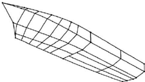
**Figure 8** – *Grid definition and resulting hull form for mono-hull vessel*
