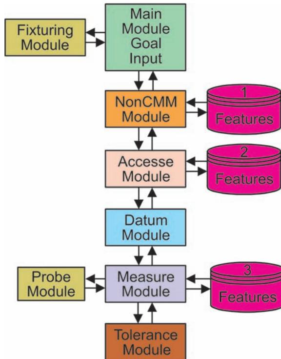
**Figure 4** – *Inspection Planning System Model*
